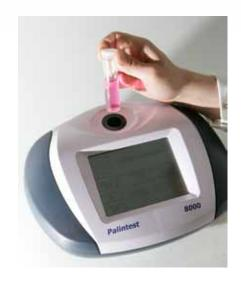
The Photometer 8000 is fully software driven, with a large backlit touch-screen providing easy access to all instrument functions. The software includes a rapid self-test of the complete instrument including the innovative optical system. The diagnostics continue to run in a permanent monitoring mode to check power supply, light levels and system integrity, reporting to the user immediately any variation that would affect the analysis.
